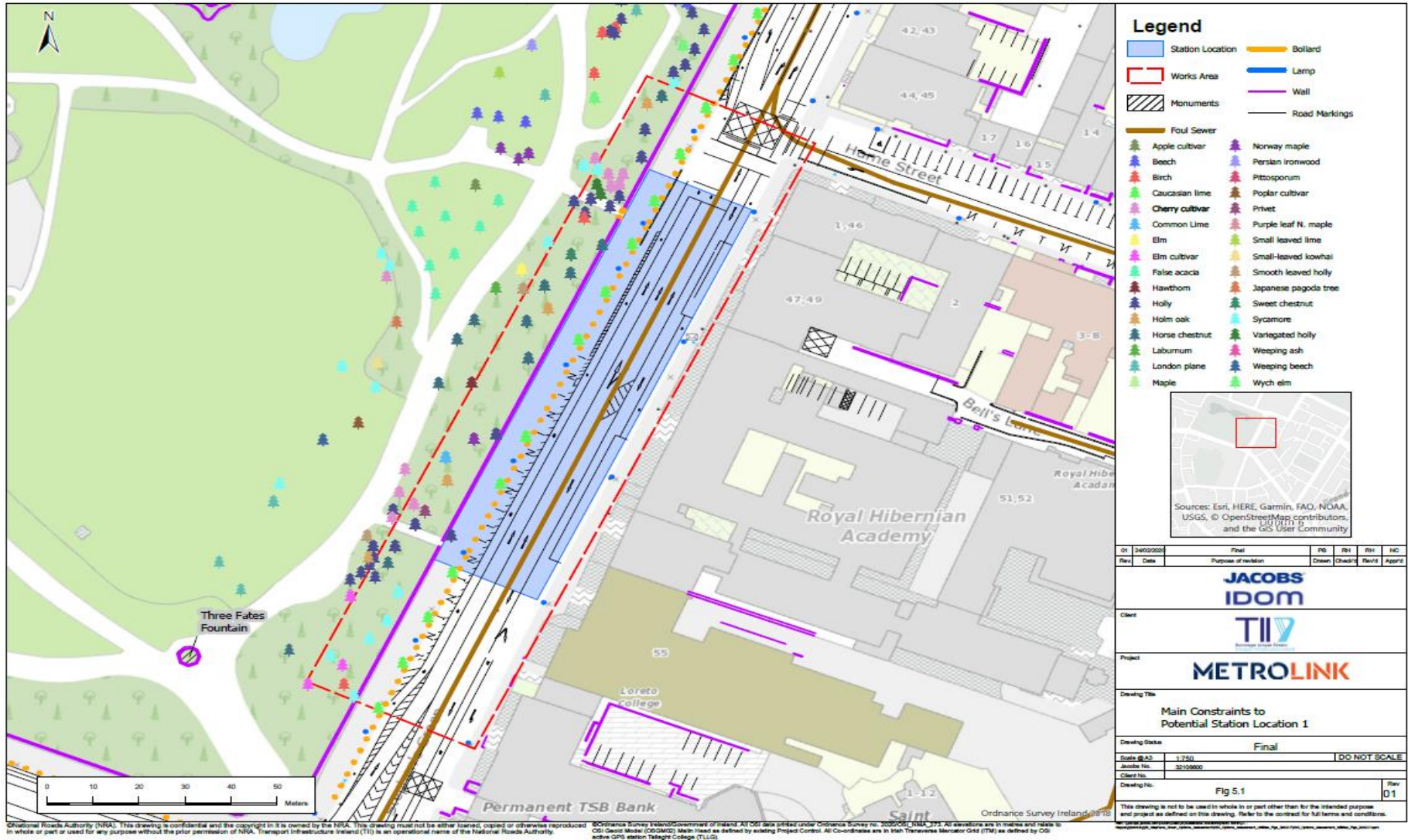
Figure 5.1: Main Constraints to potential location 1
